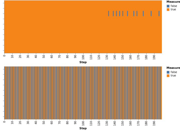
Figure 3. Comparison of the measurement behaviour of Dueling DQN on Cartpole environments with cost of 0 (top) and 0.3 (bottom). The show that when the cost is greater than zero, the agent learns to measure only when necessary to achieve the goal.
